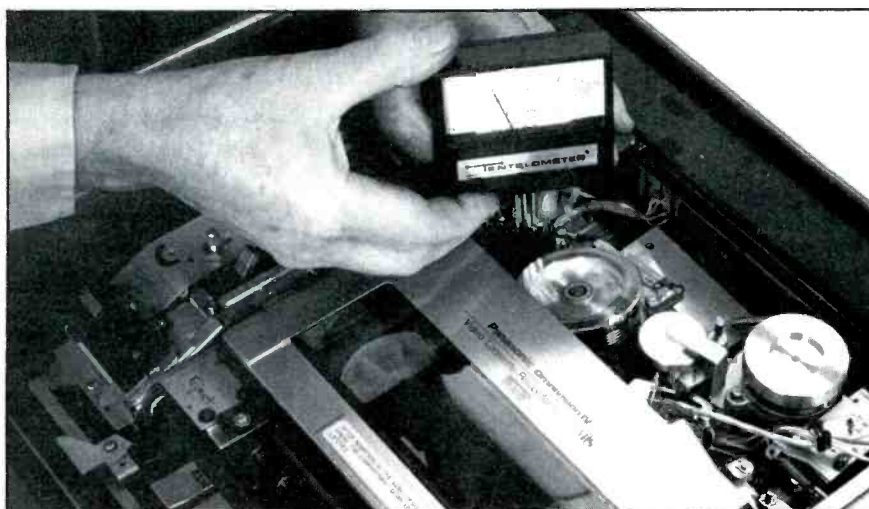
Back tension may be adjusted using a Tentelometer. Tension should be in the range of 30 \pm 5 grams.
