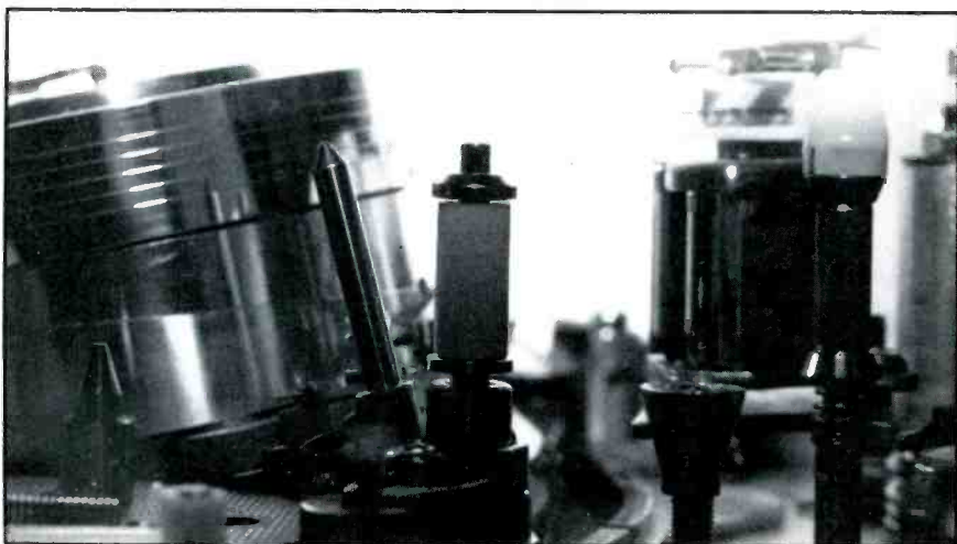
Guide posts such as this help keep the tape in proper position.
