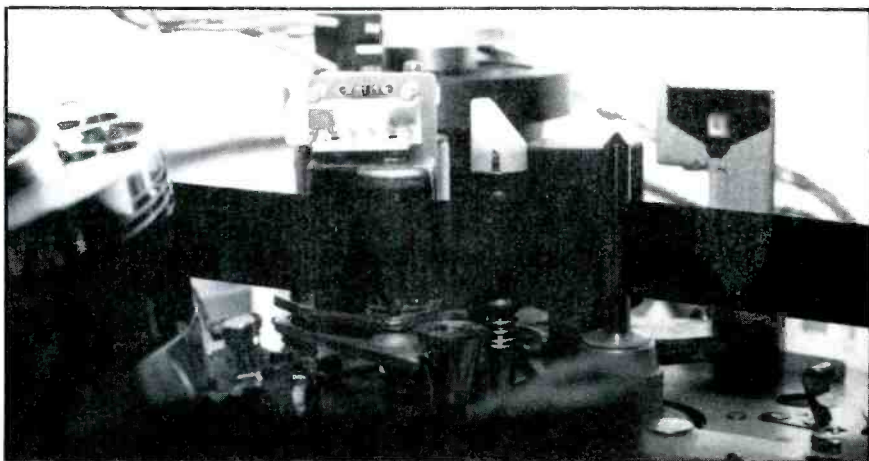
After the tape leaves the record/playback heads (upper cylinder) it encounters the CTL/audio head.
